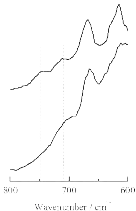
Fig. 12. FT-IR spectra of natural abundance control (a) and SEF7 crystallized by the removal of FB (b).
