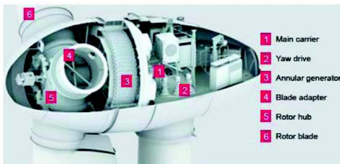
Cross sectional drawing of nacelle E-82 E2 / 2,300 kW
